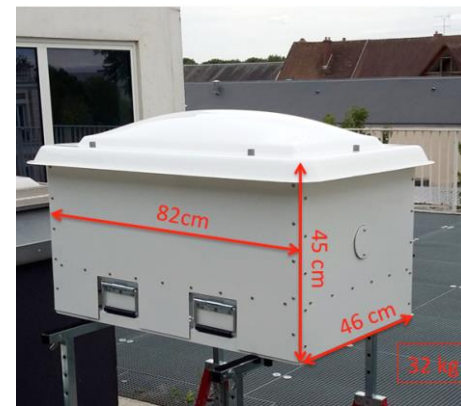
mini-BASTA (LATMOS) 94 GHz, scanning
